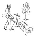
Keep a good balance and a firm foothold. Do not overreach. Keep proper footing and balance at all times.
