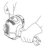
**CAUTION!** Do not pull the starter cord all the way out and do not let go of the starter handle when the cord is fully extended. This can damage the machine.
